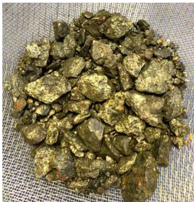
Example of sulphide mineralisation encountered in drilling at Trafalgar (HMTRRC001, 151-152m (refer ASX announcement 20 January 2021))
