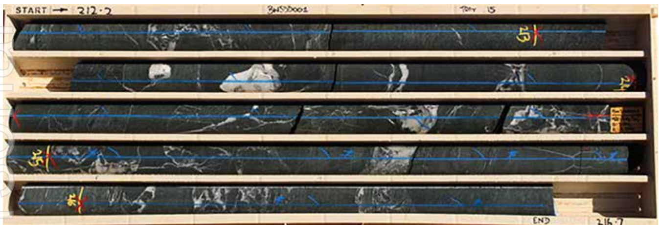
BWSDD001 212.2-216.7m. The core shows the vein styles and alteration accompanying mineralisation at Bronzewing South. This zone is accompanied by fine grained disseminated pyrite. (see ASX announcement 15 January 2021)
