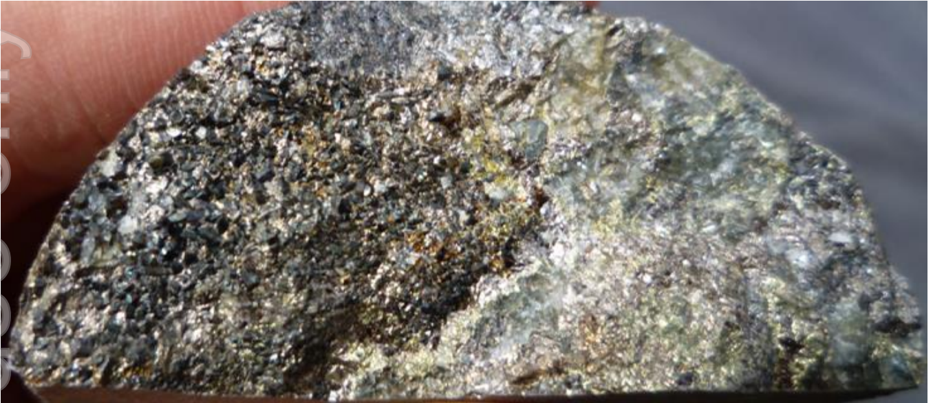
Figure 7 | Photo of coarse grained cassiterite on the left hand side, in drill core from 174m in ML134
