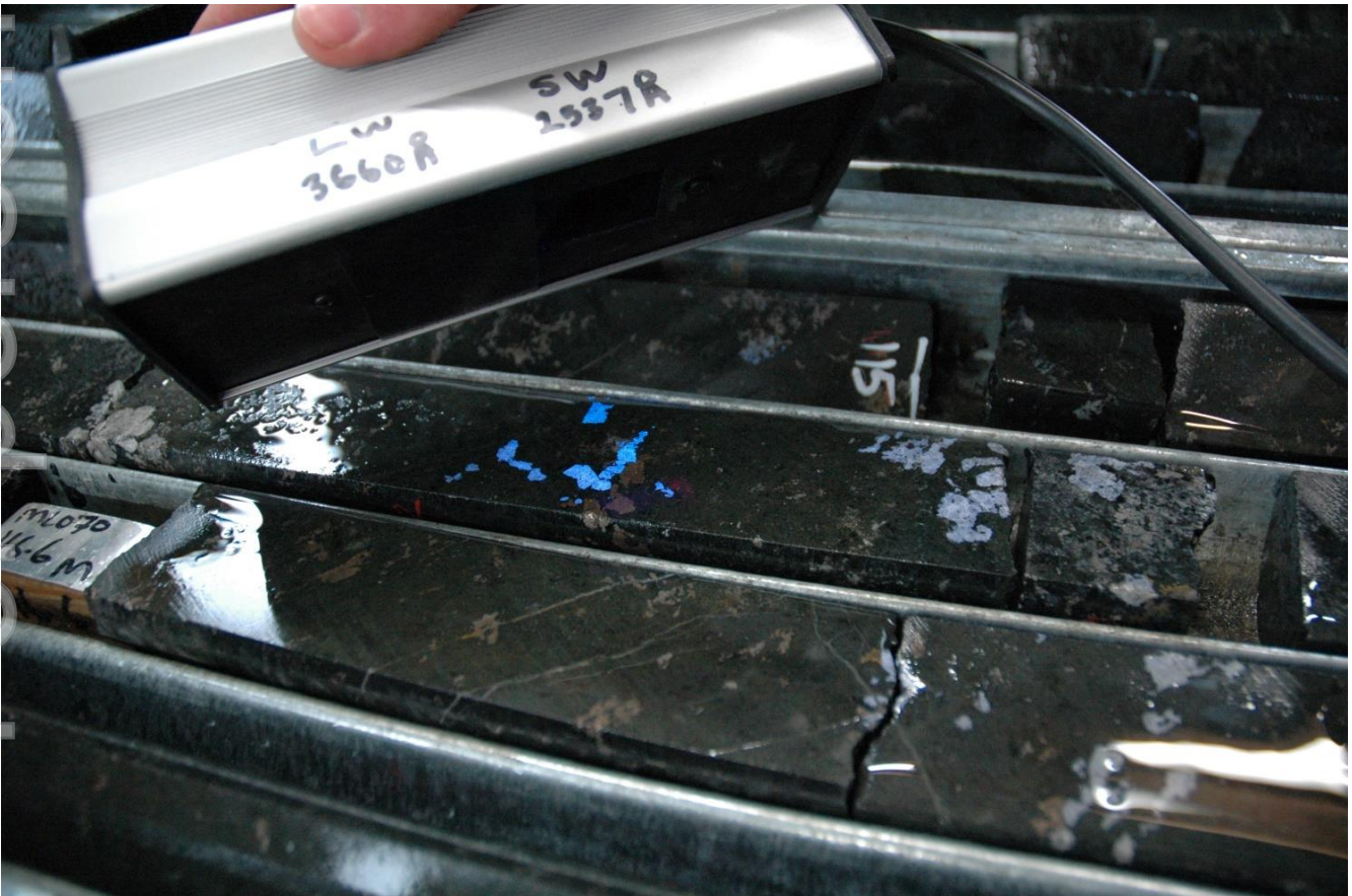
Figure 8 | Photo of scheelite glowing blue under short wave ultraviolet light in drill core from 116m in ML070
