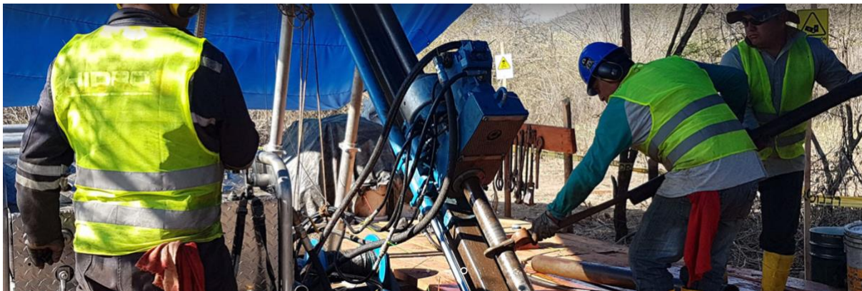
Figure 3: Drill crews operating a man portable diamond rig at Cerro Verde Prospect, Dynasty Project.
