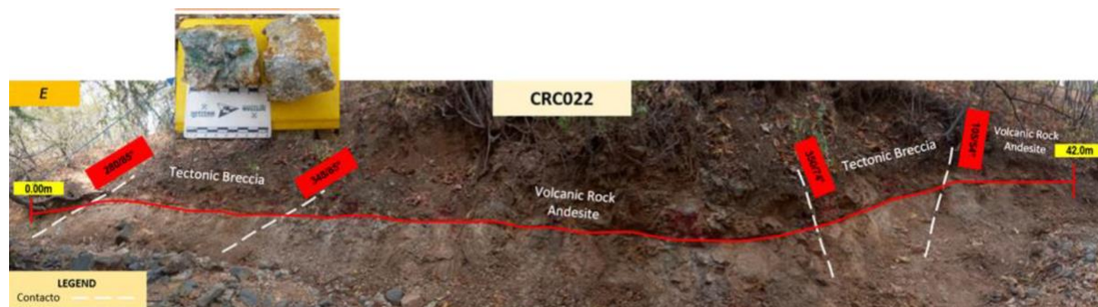
Figure 4: Photo of Channel sample CRC022 returning 42m @ 0.31% copper with 0.12g/t gold hosted in Andesite volcanics and peak value of 0.54% copper in tectonic breccia.
