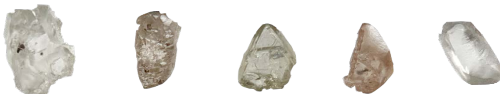
Photo (from left to right): 0.93, 0.59, 0.49, 0.41 and 0.30 carat diamonds recovered from L028 kimberlite bulk sample
