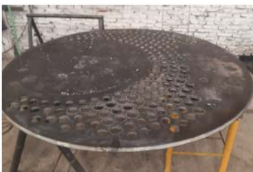
Figure 4. Rincon Lithium Project – 2,000tpa Operation Fabrication Works (Industrial Boilers)
