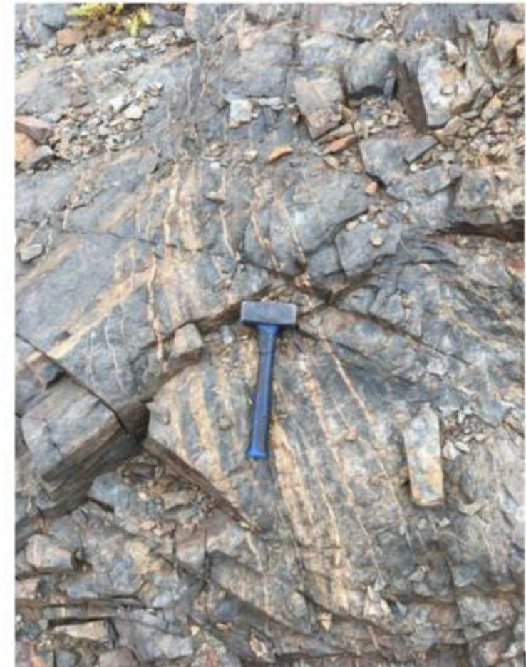
El Zorro – Au bearing sheeted quartz veins in sediment
