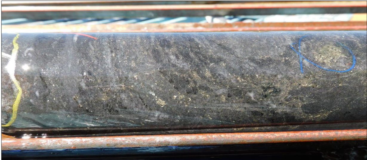
Figure 2: Fine-grained garnet-bearing mafic volcanic/sedimentary (country rock) near the contact of the mafic-ultramafic intrusion with copper sulphides and pyrite at 454m down-hole in Hole 2. Large garnet megacrysts (not in photo) also appears to be a focus point for copper sulphide mineralisation.
