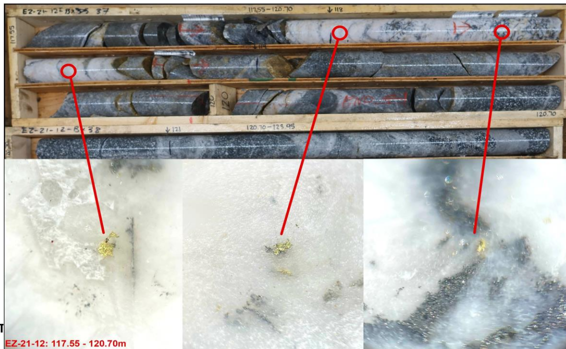
Figure 4 – EZ-21-12 drill core showing visible gold
