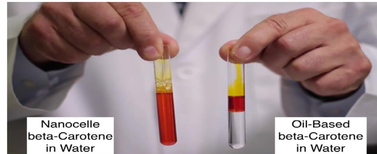
Figure 2a: NanoCelle™ fat-soluble beta-carotene (left) dispersed and soluble in an aqueous phase versus fat-soluble beta-carotene (right) insoluble in water sits on the surface of water phase.
