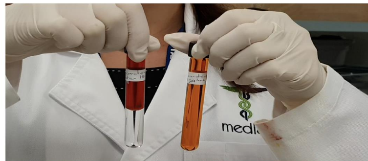
Figure 3b: NanoCelle™ fat-soluble beta-carotene at a concentration of 1.5 mg/mL (right) dispersed and soluble in an aqueous phase versus fat-soluble beta-carotene (left) insoluble in water sits on the surface of the water phase.
