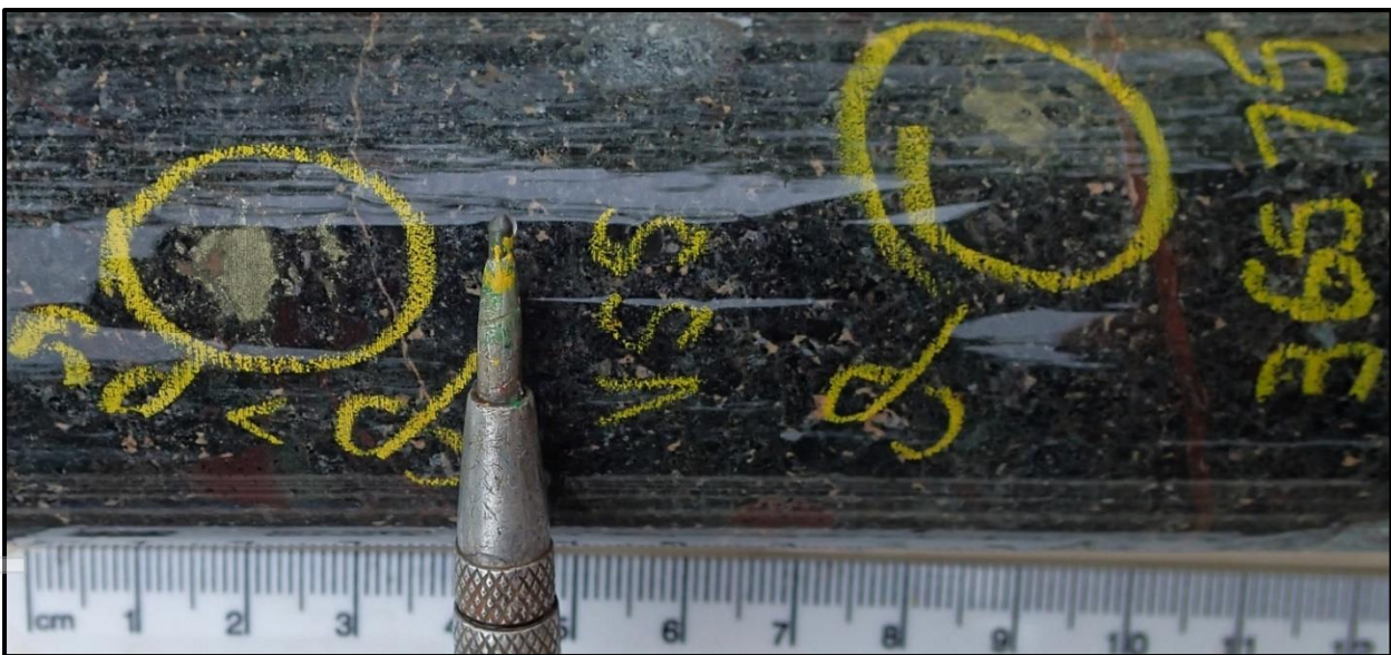
Figure 3: Coarse-grained blebby chalcopyrite and lesser pyrite at 365.75 metres in a chloritic volcaniclastic sandstone hostrock in SDD001. (Ruler for scale in cm)
