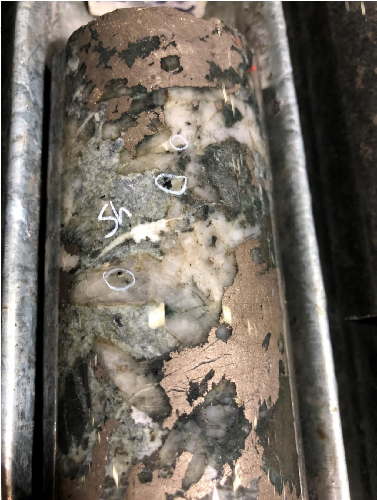
Figure Two | Photo of mineralised skarn at 119.9 m in ML339M (Sh = Scheelite)
