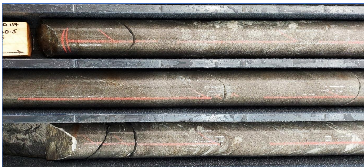
Figure 2: Folded graphite-pyrrhotite rich metapelite (RB_B target conductive source, 21AFDD117, ~440m)
