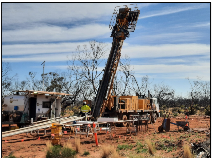
Figure 1 – Diamond drilling at the Delta Blues prospect in the Fraser Range
