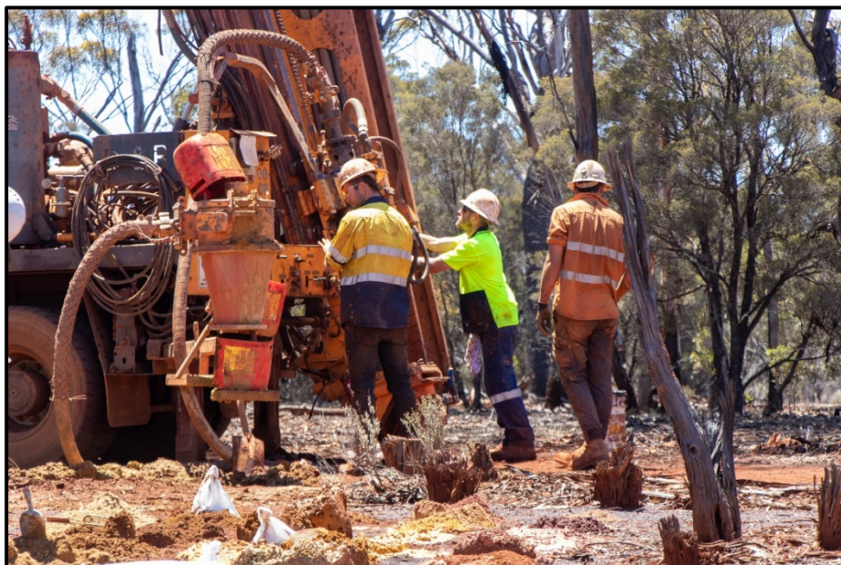
Figure 1 – Aircore drilling at Galileo's Norseman project.
