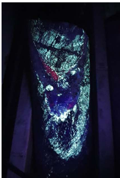
Core in UV light with tin-bearing malayaite fluorescing green.
