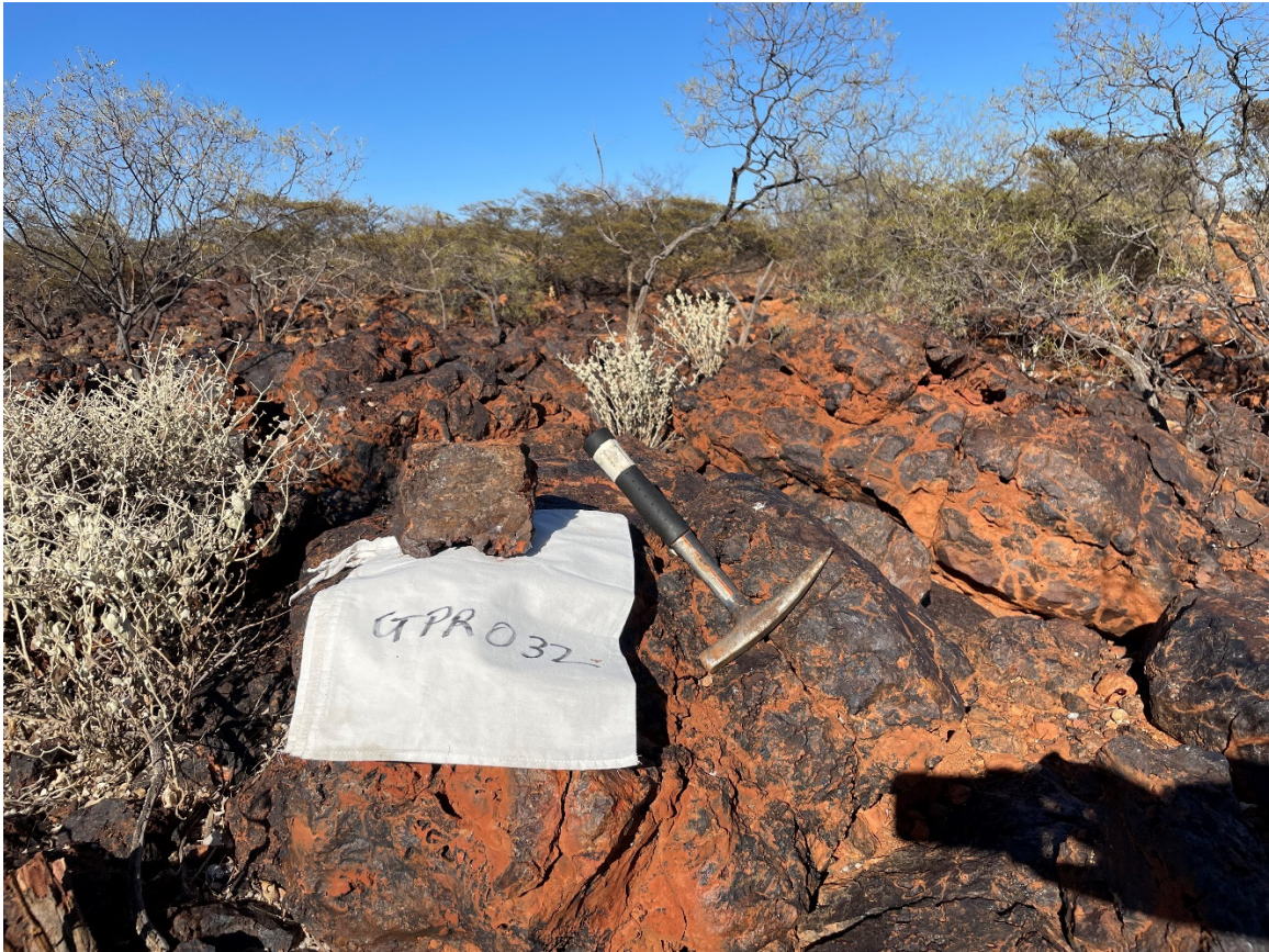
Figure 2. Additional sampling at ironstone discovered at Lyon_11 Prospect, which returned 4800ppm TREO in reconnaissance sampling, with the aim to identify if higher grade Neodymium and Praseodymium is present.
