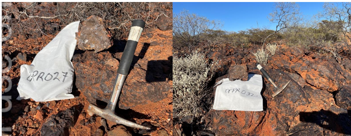
Figure 2. High-grade ironstone at Lyon_11 prospect returning a peak of 8.01% TREO, above samples GPR027 (2.07% TREO) and sample GRP032 (3.05% TREO)
