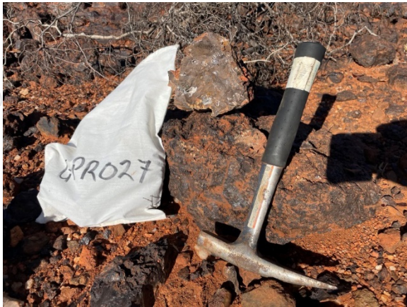
Figure 7. High-grade ironstone at Lyon_11 prospect returning a peak of 8.01% TREO, above samples GPR027 (2.07% TREO) and sample GPR032 (3.05% TREO) Mineralogy.
