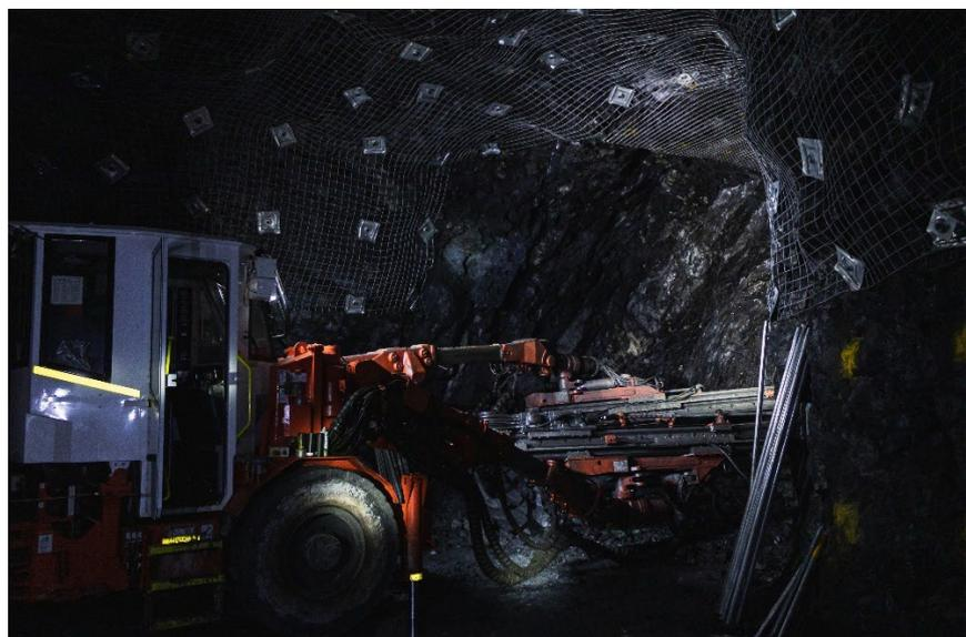
Figure 1. Jumbo undertaking meshing and bolting at Avebury.
