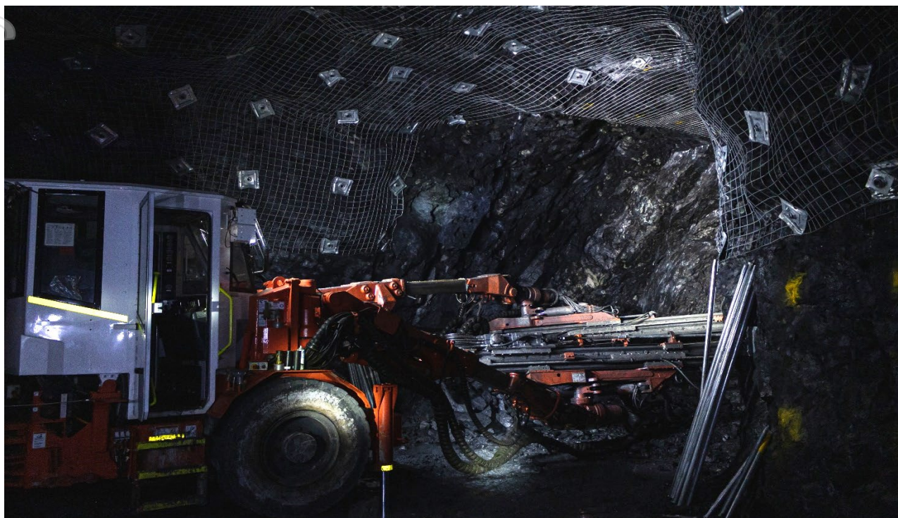
Figure 4. Jumbo undertaking underground development drilling.
