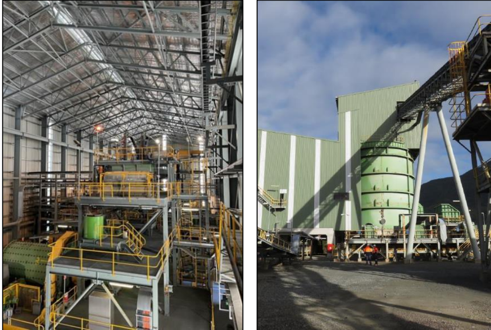
Figure 12: Plant infrastructure – grinding and flotation circuits (left); crusher house and fine ore bin (right) Source: Mallee Investor Presentation June 2022
