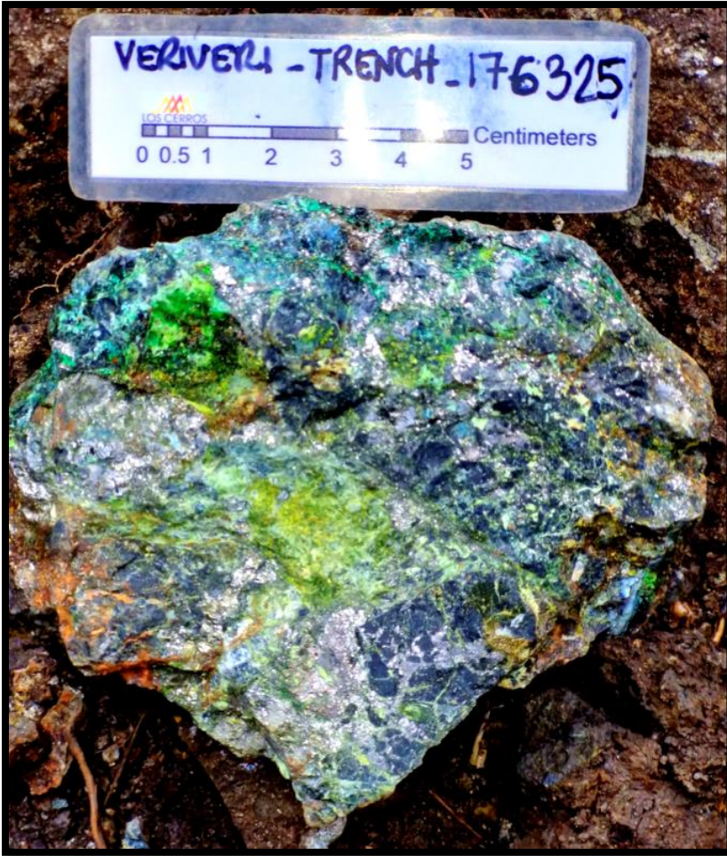
Plate 1. Representative photo of trench sample 176325 which returned 10.86% Ni, 2.12 g/t Au from 135-136m. The sample contains nickel sulphide (heazlewoodite), serpentine and garnierite.
