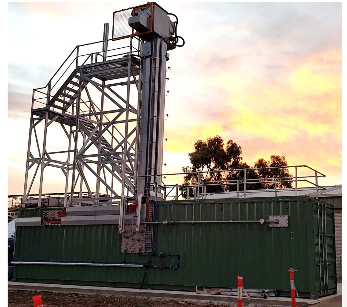
Direct electrical heating has been proven at pilot scale at the Calix Technology Centre.
