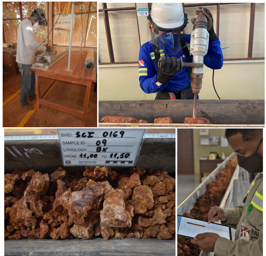
Figure 26 Photographic documentation of the core sample cover removal, crumbling, intervals splitting and logging
