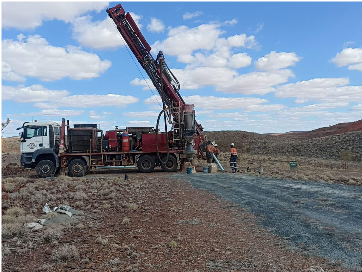
Figure 2 RC Drilling at Tambourah King.
