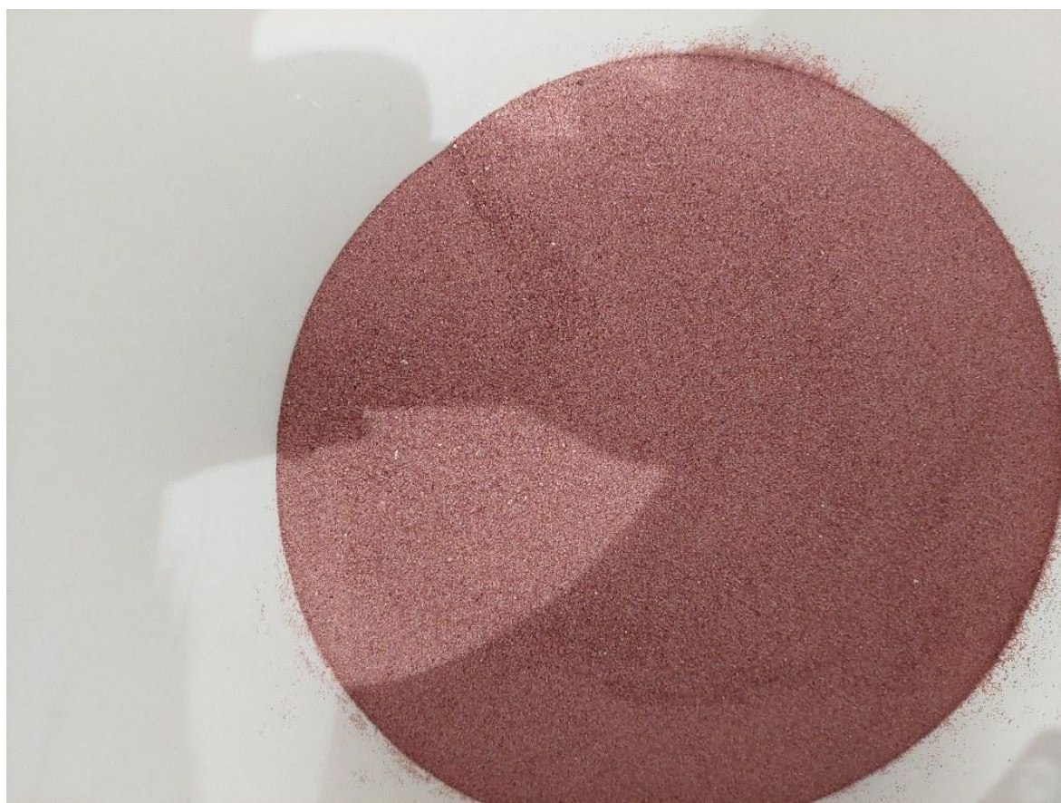
Figure 10: Coarse alluvial almandine garnet product produced during bulk metallurgical test work
