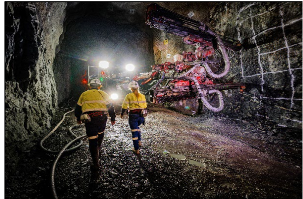
Figure 2: Jumbo development in Mt Mann orebody
