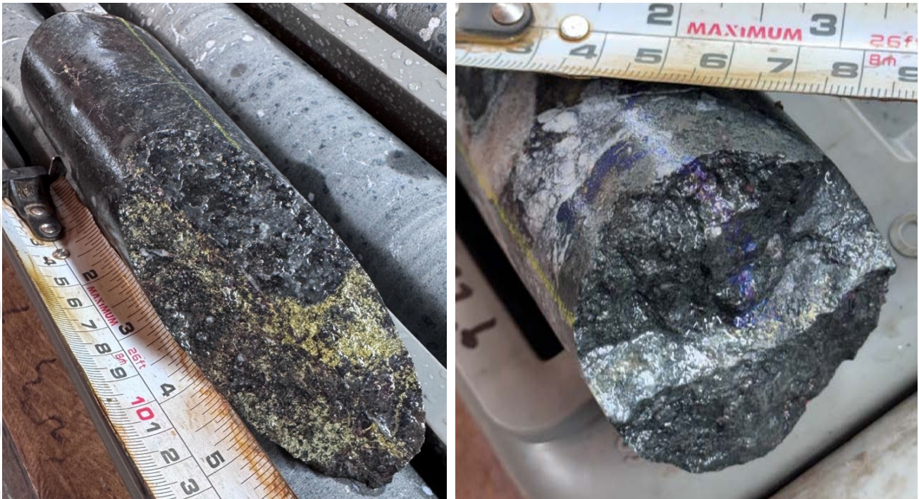
Figure 7 - Example of chalcopyrite mineralisation (left) and bornite-chalcopyrite mineralisation (right) from 230.5-233.34m downhole in DAN26030.
