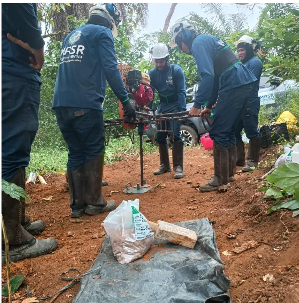
Figure 1: Auger drilling at one of the priority locations for the Campo Grande Project.
