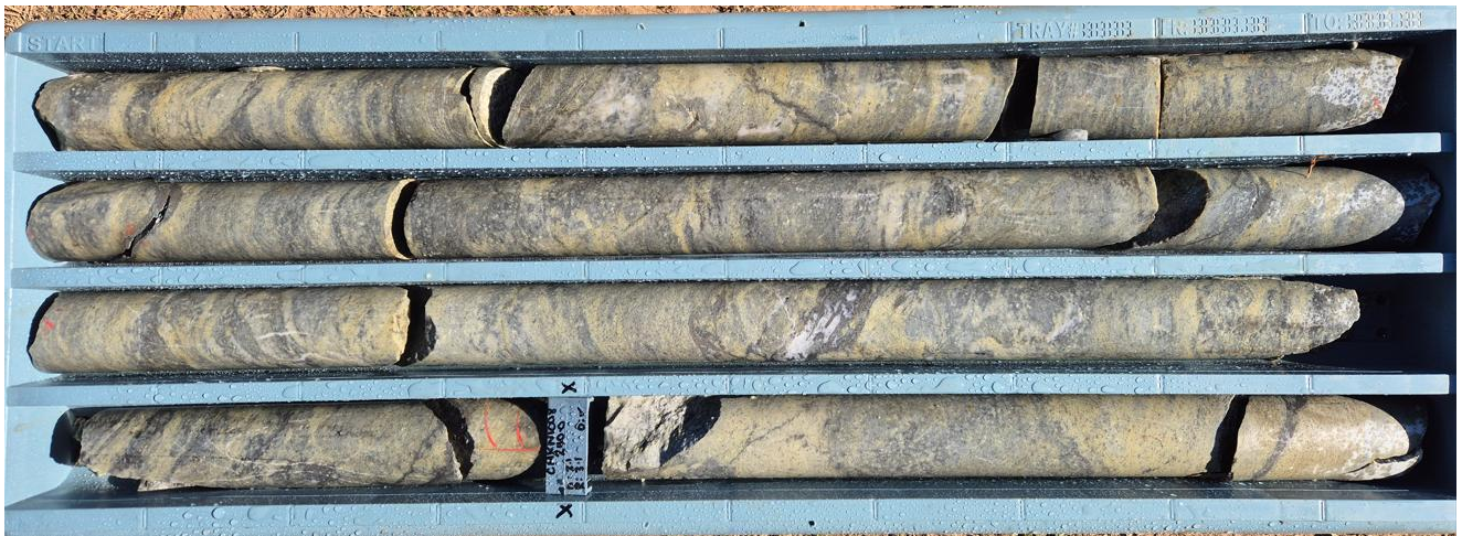
Figure 2: Diamond drill core (HQ) from hole CMKNI008 showing stockwork style arsenopyrite-pyrite-proustite stringer veins within sericite-altered rhyolite porphyry.
