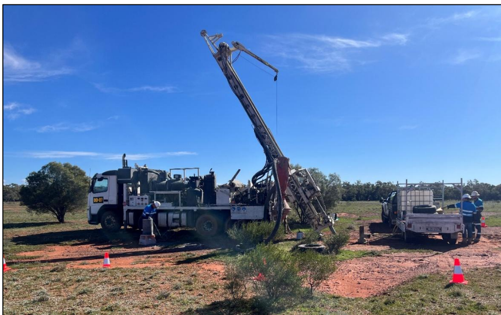
Figure 1: AC Drilling underway at the Blind Freddie Prospect
