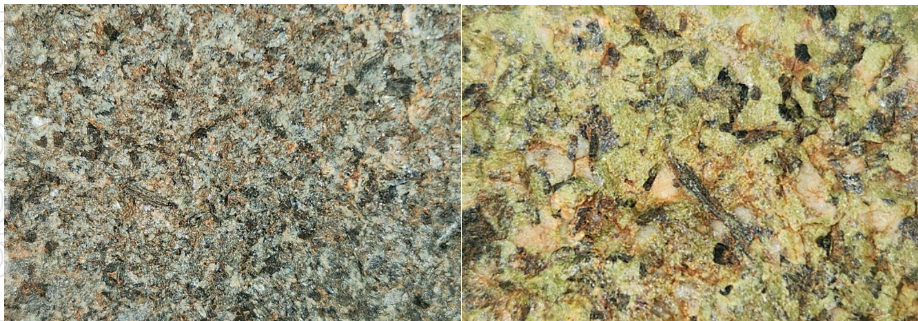
Figure 5. Olivine gabbro (left) and serpentinite rich in augite and lizardite-antigorite (right).
