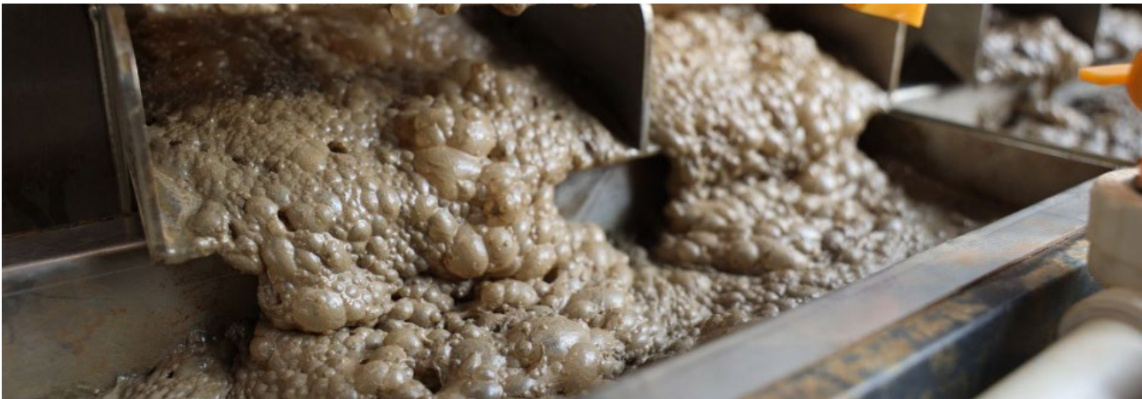
Figure 32: Froth Formation During Pilot-Scale Flotation Testwork
