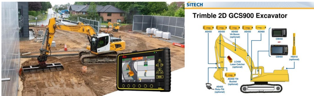
Figure 23: Indicative High-Precision GPS Excavator Machine-Guidance System.
