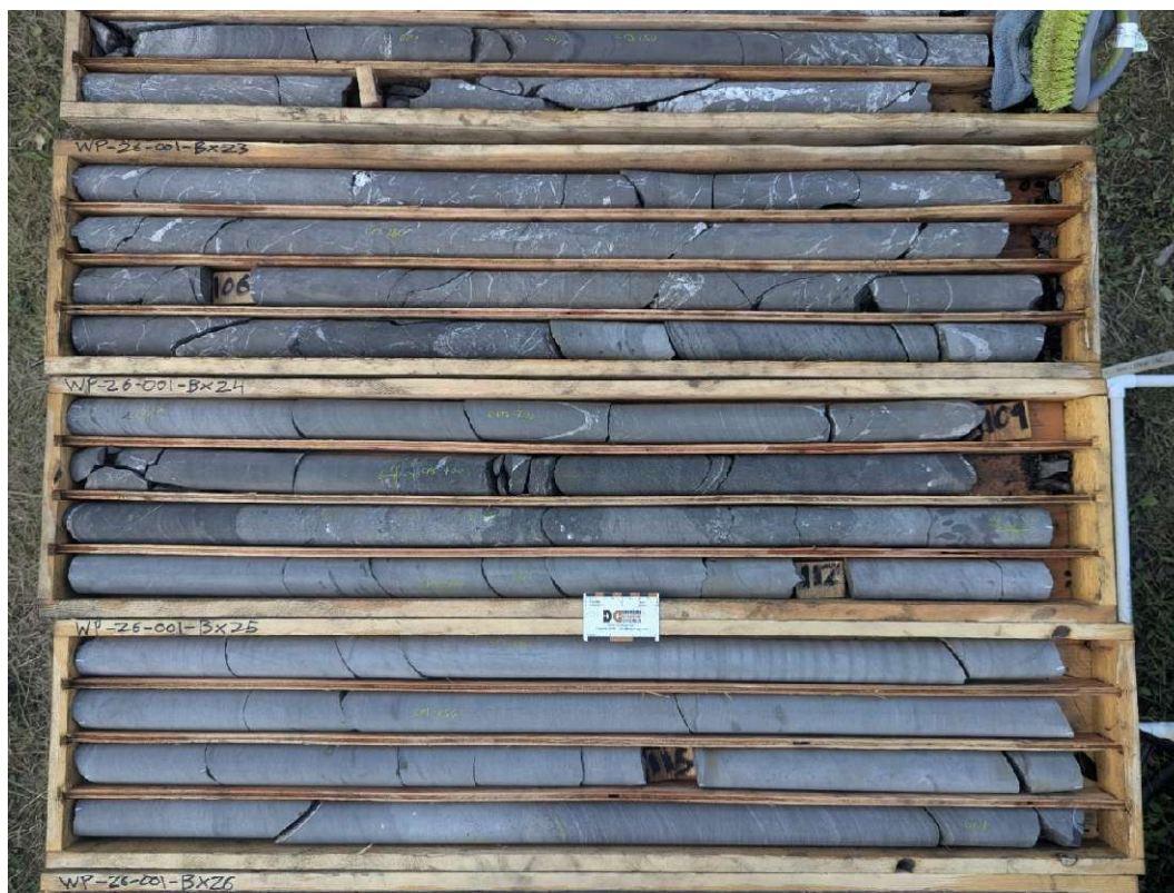
Figure 1: WP26-001 drill core displaying interpreted Main Zone intersection (based on visual logging only and is not assay confirmed)
