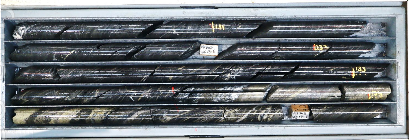
Figure 3. MZS43 133.5 – 134.5m. 1.0m of massive jamesonite (Sb sulphide) - pyrite - arsenopyrite – tetrahedrite (Ag sulphide) mineralisation (Hanging wall Lode).
