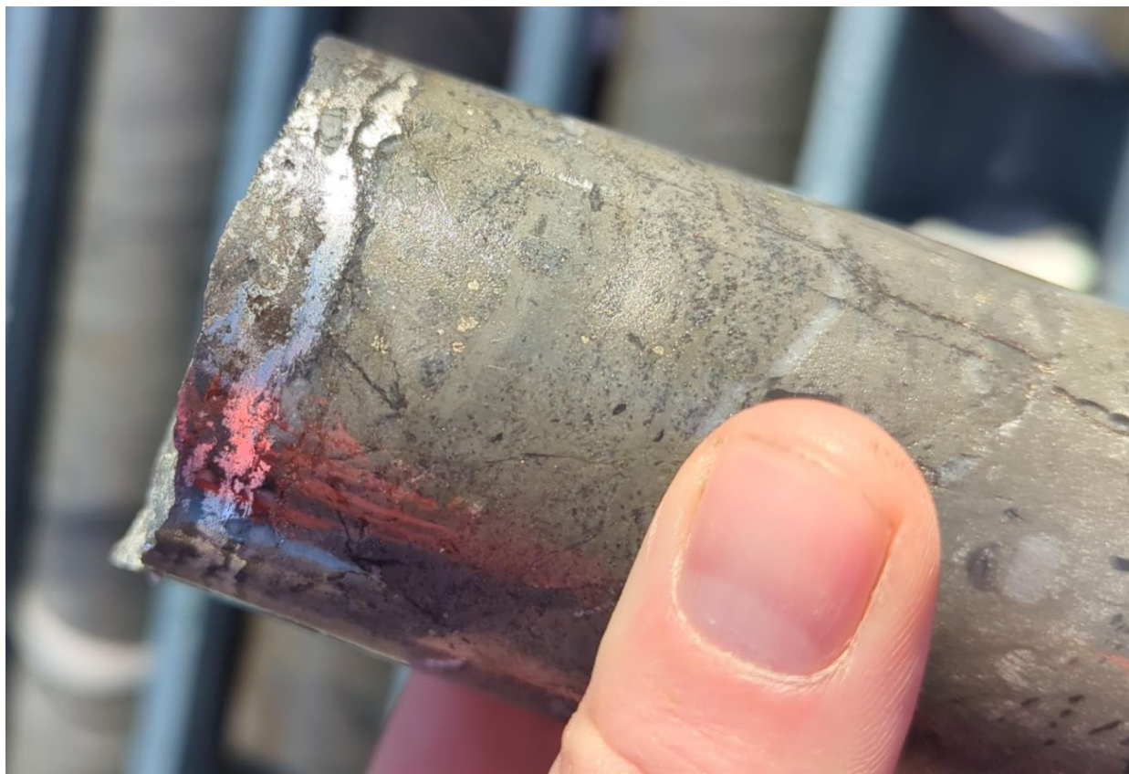
Figure 8. Vein containing a significant volume of native antimony metal (metallic white) intercepted in CSK045W1 (538.15m). The vein also contained stibnite and pyrrhotite, and pyrite wallrock alteration can be seen in the image. Please refer to Appendix 1 for the relevant assay results relating to Figure 8.
