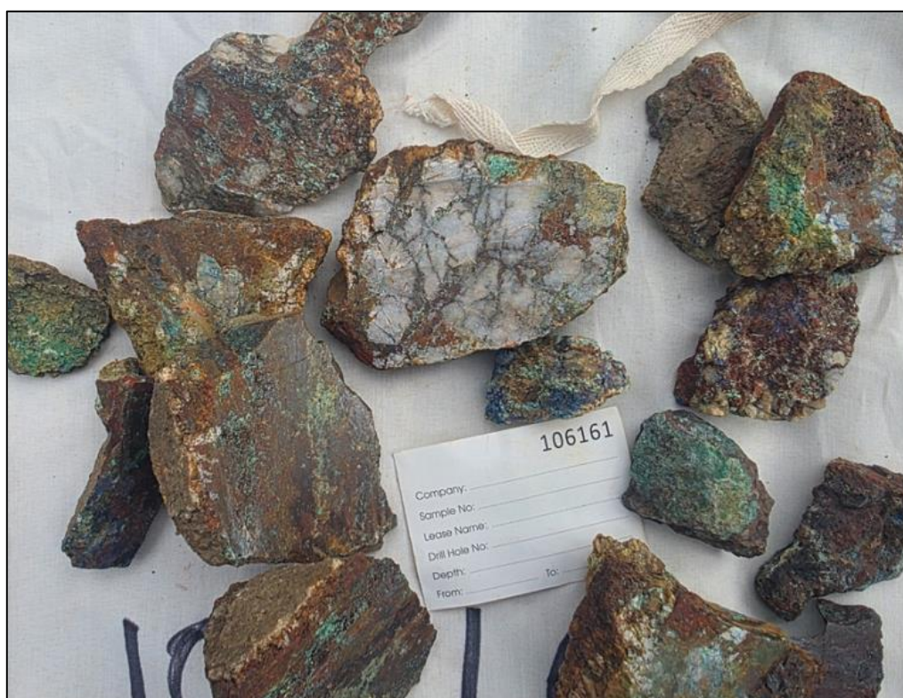
Figure 4: Sample No: 106161. FOV 25 cms. Location: 189992mE 8028064mN. Brecciated milky white vein quartz infilled by limonite coated by ubiquitous malachite and uncommon azurite. No observable wolframite. Estimate <1.00% W. Assay: 2.22ppm Au, 0.21% Sn, 1.31% W
