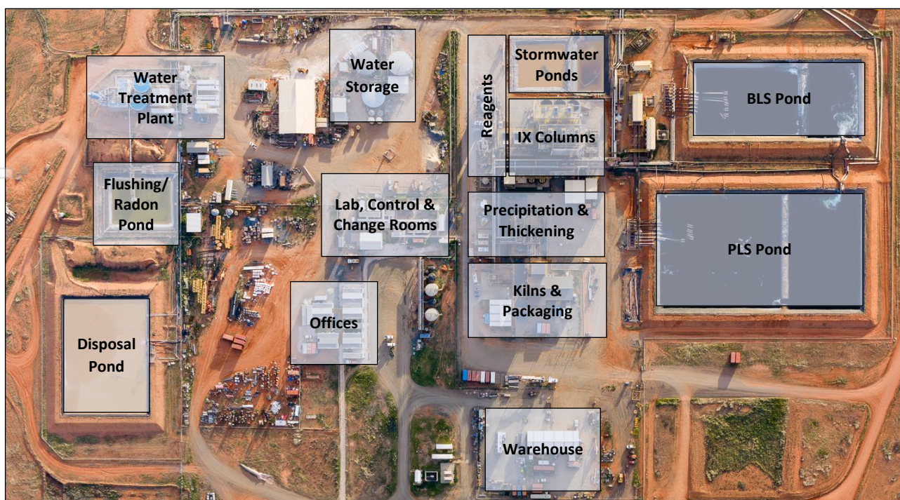
Figure 28: Overview of existing process plant areas at Honeymoon
