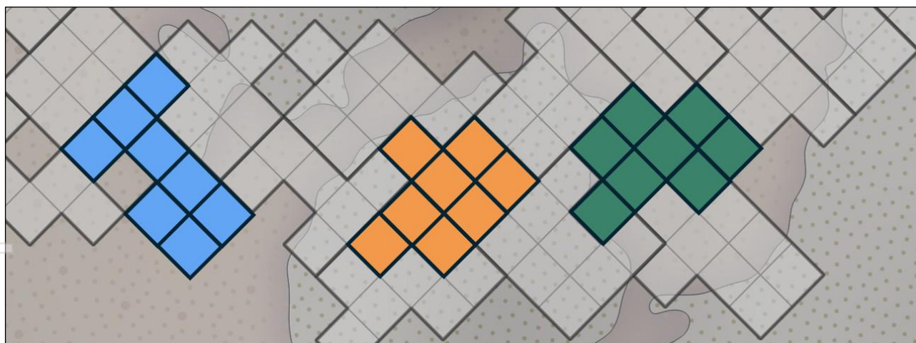
Figure 26: Typical grouped 8 pattern wellfield layouts used for infrastructure planning and assessment. Each highlighted square represents a five-spot pattern consisting of an extraction well at its centre and an injection well at each of its corners. Corresponding colours represent grouping into 8 pattern sets to be serviced by a single 8-pump wellhouse.
