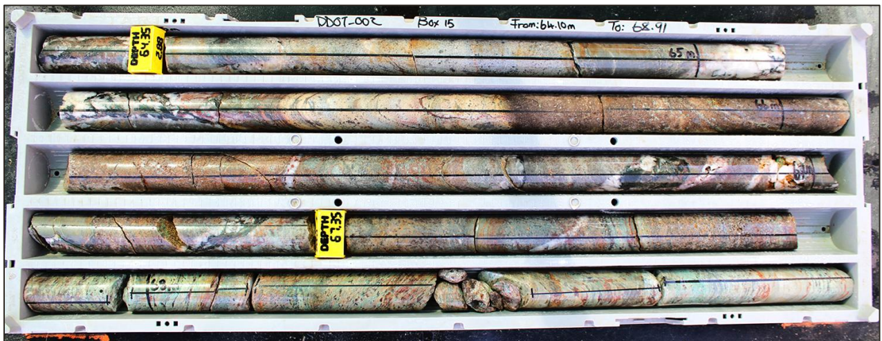
Figure 1 - DDOT002 Core from 68.13m to 68.34m showing disseminated malachite, chrysocolla, cuprite and chalcocite mineralisation (left) and DDOT001 Core from 64.03m to 64.17m showing disseminated chalcocite, cuprite and diopside mineralisation (right). Refer to Appendix A for details of visual estimates of mineralisation.
