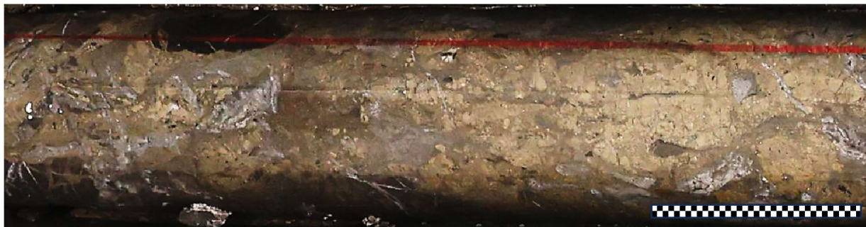
Figure 5. CD26-013 at 292.6m; Brecciated semi massive sulphides showing sulphide replacement of some clasts. The dark green sulphides are predominantly pyrite, the yellow green to brassy-yellow sulphide is chalcopyrite, with dark clasts of unmineralised shale and with white carbonate veins. Scale bar approx. 5cm
