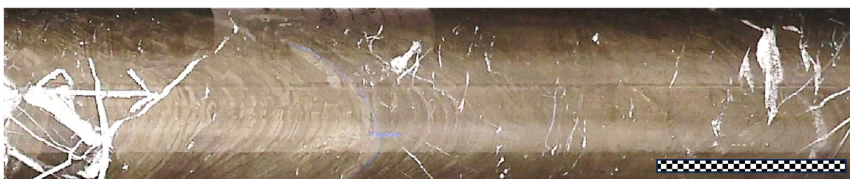
Figure 4. CD26-013 at 182.7m; laminated massive sulphides. The dark green sulphides are predominantly pyrite, the yellow green to brassy-yellow sulphide is chalcopyrite, with white carbonate veins. Scale bar approx. 5cm
