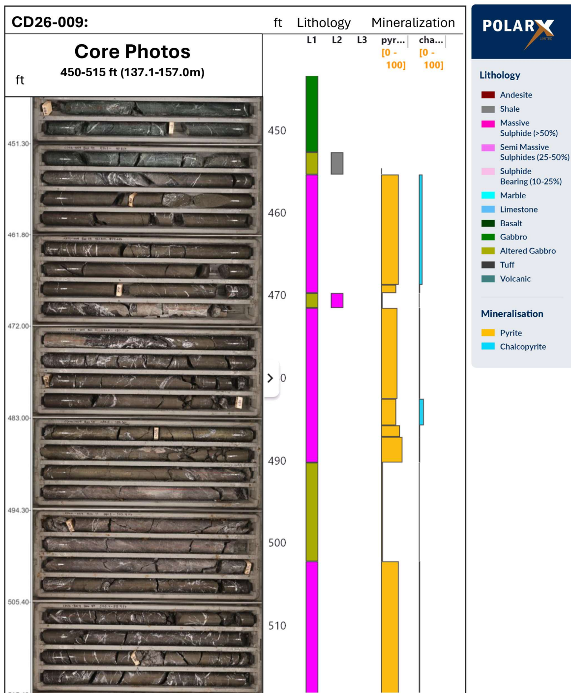
Figure 10. Core photos, associated lithologies and estimated logged chalcopyrite (cha) and pyrite (pyr) percentages for CD26-009
