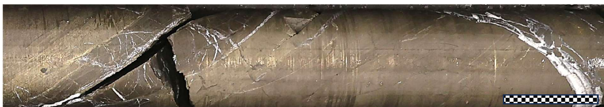
Figure 3. CD26-009 at 194.7m; massive sulphides. The darker sulphides are predominantly pyrite, the yellow green to brassy-yellow sulphide is chalcopyrite, with white carbonate veins. Scale bar approx. 5cm
