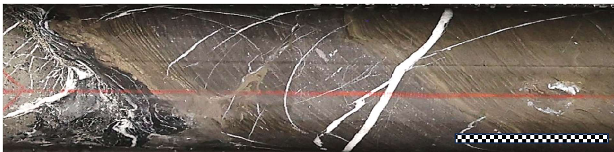
Figure 2. CD26-009 at 138.7m; altered gabbro grading into shale hosted laminated massive sulphides, predominant pyrite with brassy chalcopyrite thinly interbedded with white carbonate veins. Scale bar approx. 5cm
