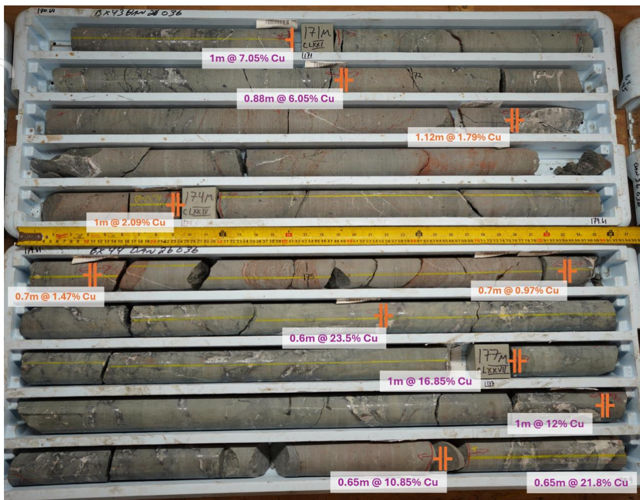
Figure 6 - Labelled photograph of key mineralised interval in drillhole DAN26036. Photograph from 170.64m to 178.90m. Sample intervals are labelled with the returned copper assay result, including up to 0.6m @ 23.5% Cu, 0.65m @ 21.8% Cu and 1.0m @ 16.85% Cu.
