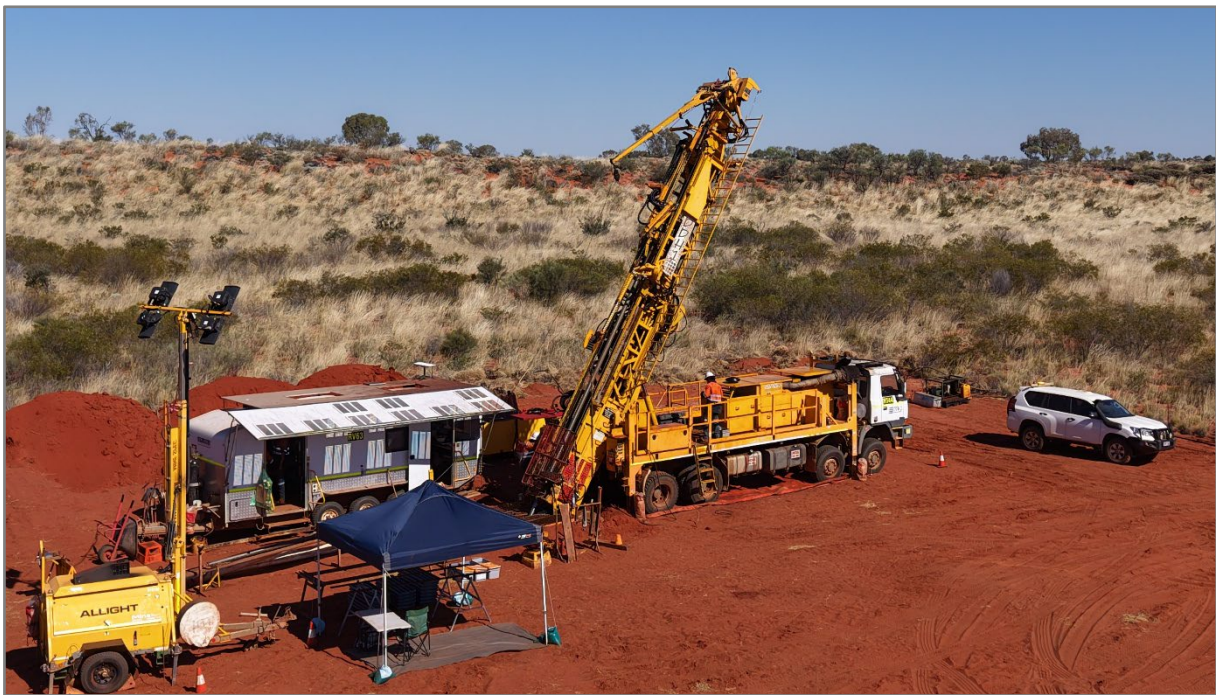
Figure 1. Diamond drilling at Khya, West Arunta Project
