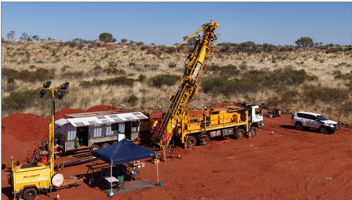
Figure 1. Diamond drilling at Khya, West Arunta Project
