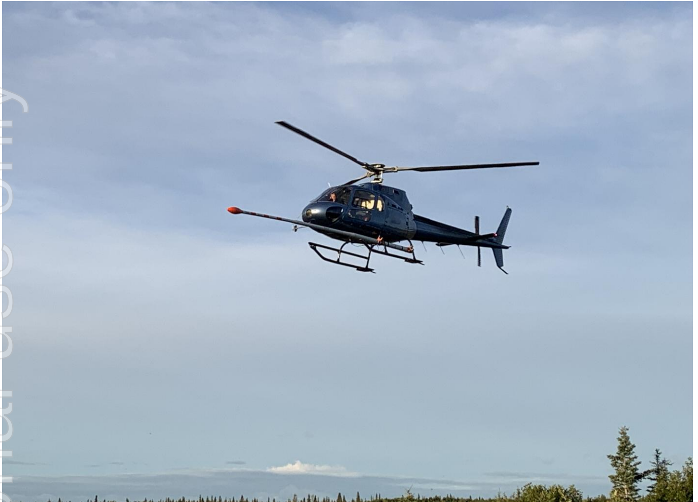
Figure 2: Commencement of geophysics survey (magnetics / radiometrics) showing Astar and survey boom
