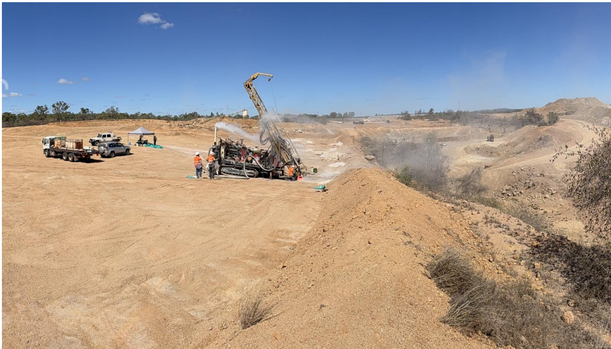
Figure 1: RC drilling underway at Blackjack North Pit, September 2026
