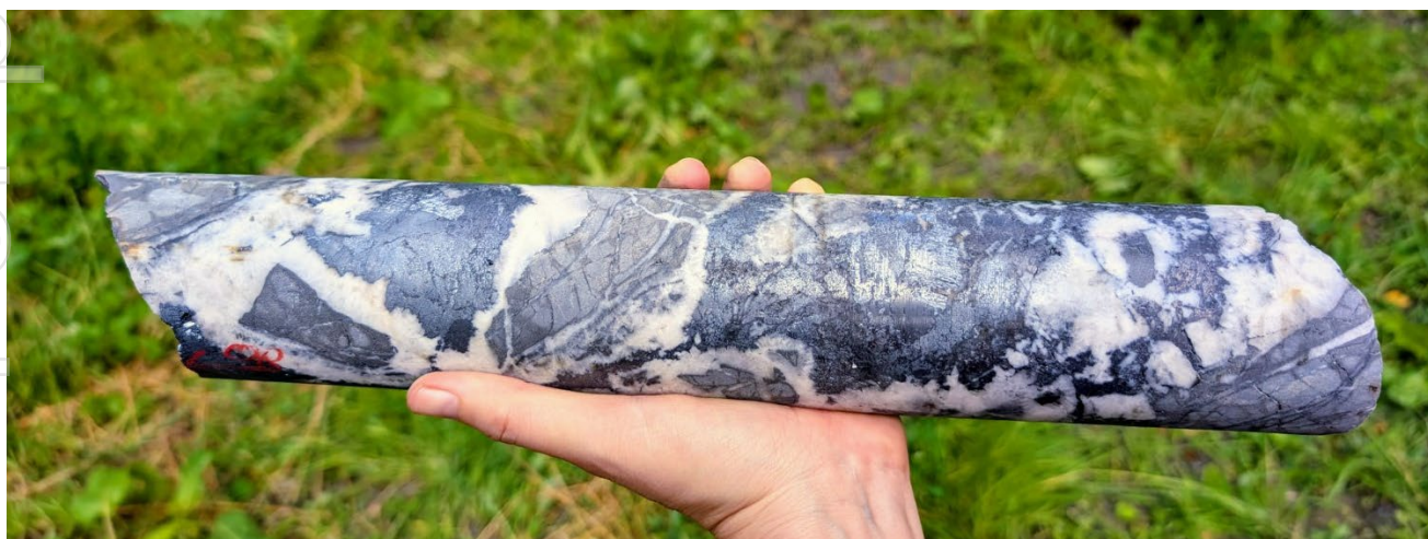
Figure 3 Photograph of 44cm long drill core from hole DD26ZOP-002 (interval 44.62 – 45.23m) which assayed at 15.3% Sb and 0.9g/t Au
