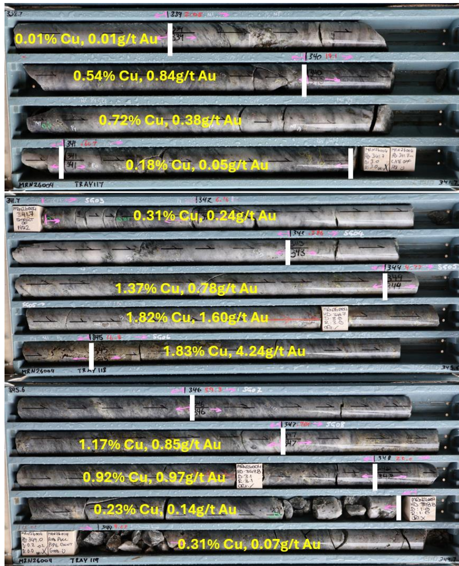
Figure 4. Primary copper mineralisation from MRN26004 with chalcopyrite (~339 – 350m downhole)
