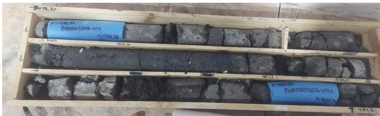
Figure 2 – DDH-3 Core Showing Brine-Bearing Lithology at Depth
