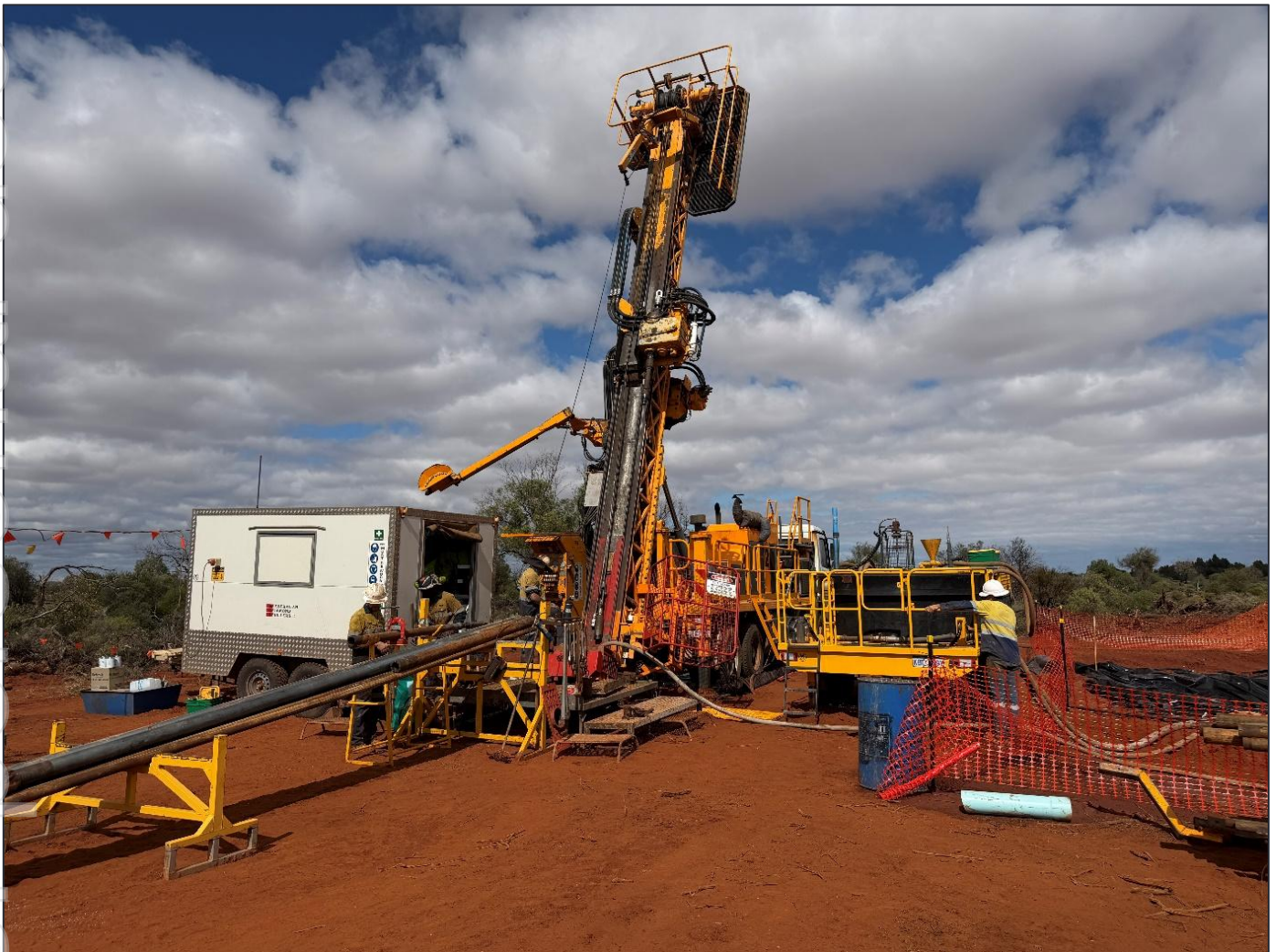
Figure 1 – Diamond drill rig setup on the Coogee North EIS co-funded drill hole, with a planned total depth of 800- 1,000m to test a major intrusive gold-copper target
